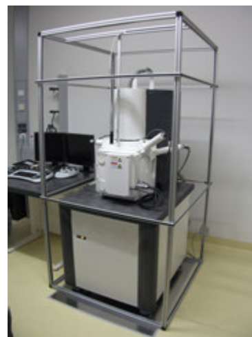
Integrated coil frame from Bilz for magnetic field compensation
