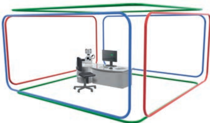
Bilz magnetic field compensation using room coils
