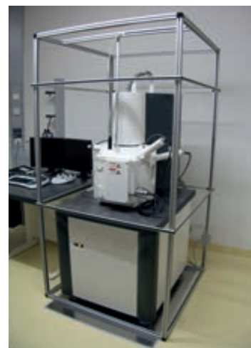
Integrated coil frame from Bilz for magnetic field compensation
