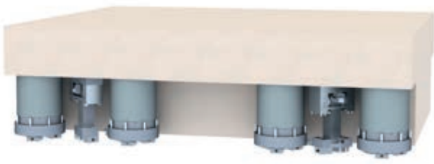
Active vibration insulation AIS™ High Performance by Bilz, which suspends the glass fibre reinforced plastic armoured foundation block weighing 75 tons on air cushions.
